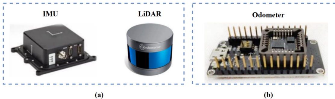
Figure 6. Sensors equipment for robot. (a) External sensors; (b) Internal sensor. IMU: inertial measurement unit; LiDAR: light detection and ranging.
