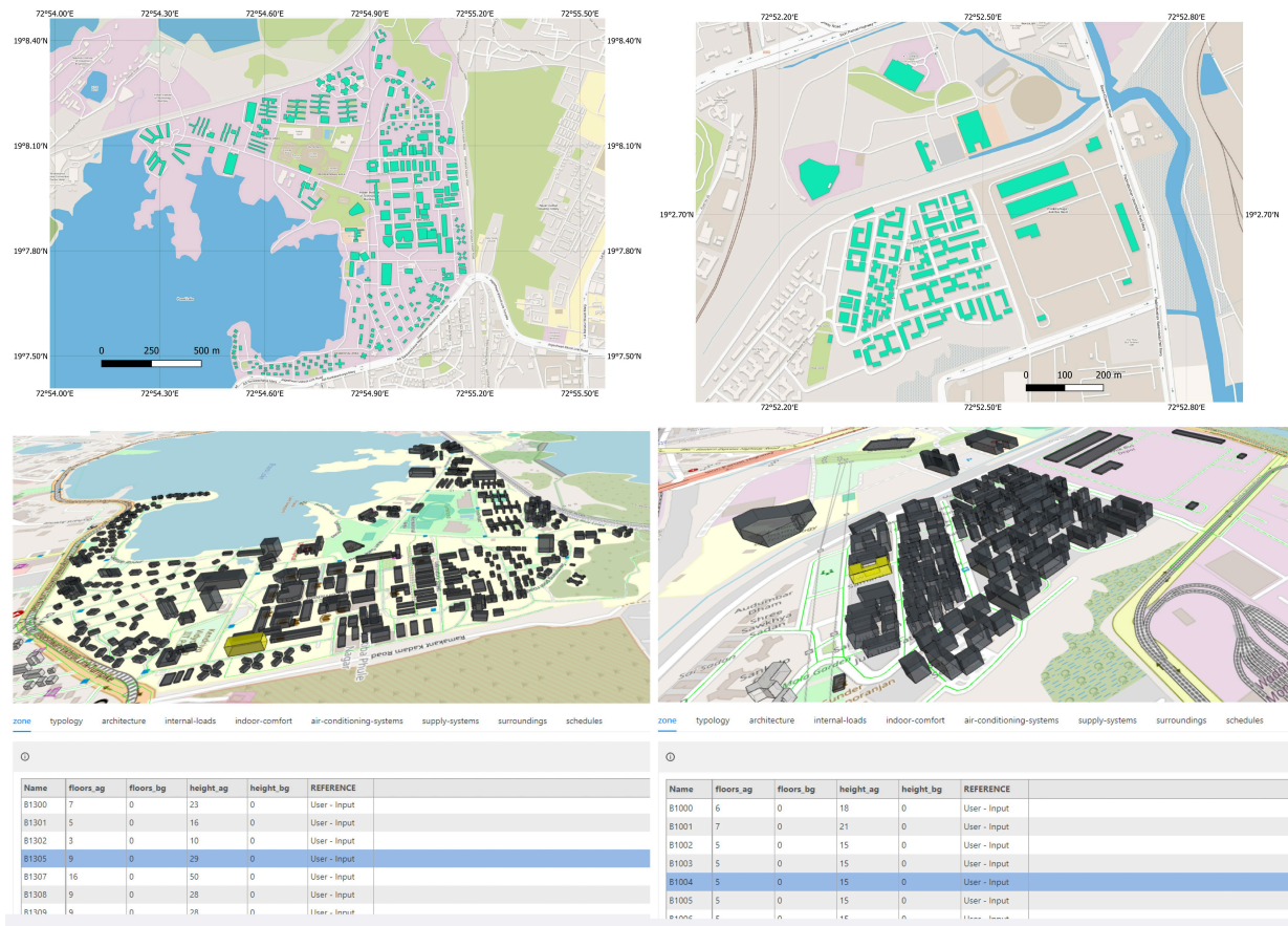
Figure 3. Building footprints and their corresponding 3D models for IIT Bombay (left) and Sion (right), with input databases pertaining to each building generated in CEA. IIT: Indian Institute of Technology; CEA: City Energy Analyst.
