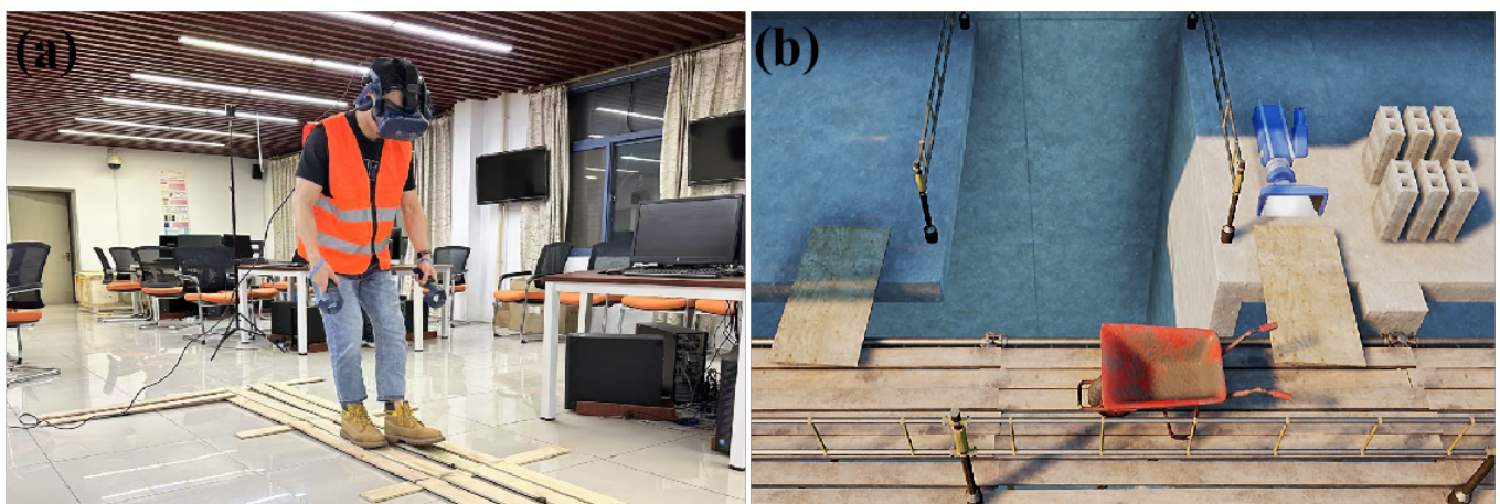
Figure 3. VR-based experiment for collecting EEG data. (a) A participant during experimental procedure; (b) VR scene layout. VR: virtual reality; EEG: electroencephalogram.
