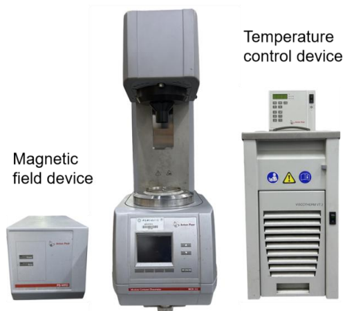
Figure S1. The on-site photos of the MCR 302 rheometer, the temperature control device and magnetic field device.
